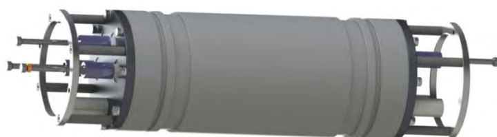
Figure 4. The Autonomous Multichannel Acoustic Recorder (AMAR; JASCO) used to measure underwater sound Geelong Harbour.
