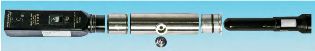
Figure C-1. Split view of a G.R.A.S. 42AC pistonphone calibrator with an M36 hydrophone.
